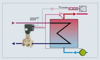
Temperature control upon input signal failure, e.g. heating
