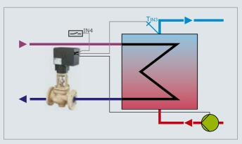
Fixed set point control with PID controller, e.g. cooling
