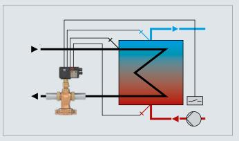
Control of the flow temperature in the secondary circuit taking into account the network supply temperature and the return flow temperature in the secondary circuit
