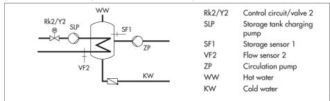
Fig. 9 · Schematics of a storage tank system with a globe valve for return flow temperature limitation
