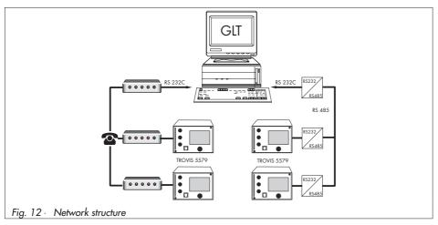
The TROVIS 5579 Controller is equipped with an RS-232 Modbus interface. Optionally, cable converters are available for operation with a four-wire (1400-7308) or two-wire bus (1400-8800).
