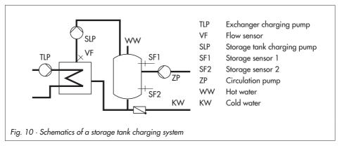
The controller begins charging the storage tank when the water temperature measured at sensor SF1 falls below the DHW temperature set point by 0.1 °C. If the flow temperature in the system exceeds the desired charging temperature, the controller tries to reduce the flow temperature in the heating circuit for up to 3 minutes before the exchanger charging pump is activated together with the storage tank charging pump.
