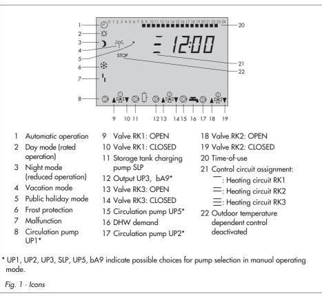
The controller status can be displayed in the operating level (-> section 1.4).
