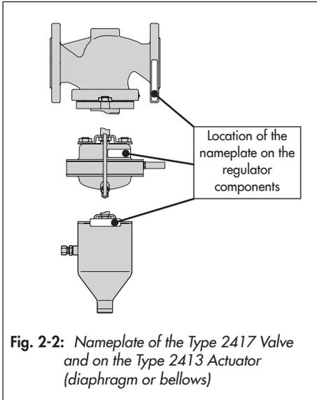
**Fig. 2-2:** Nameplate of the Type 2417 Valve and on the Type 2413 Actuator (diaphragm or bellows)
