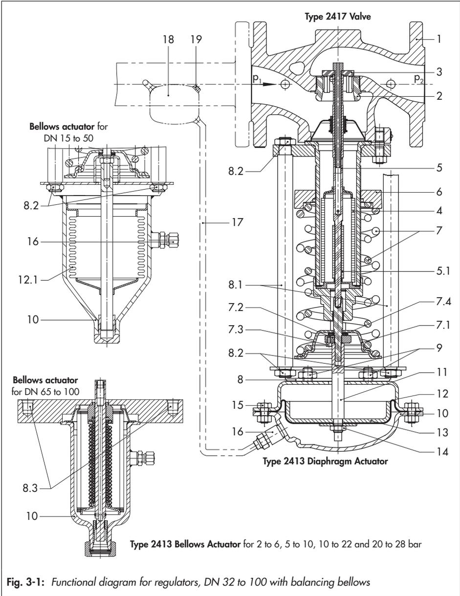
Fig. 3-1: Functional diagram for regulators, DN 32 to 100 with balancing bellows
