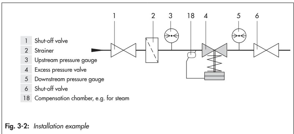
Fig. 3-2: Installation example
