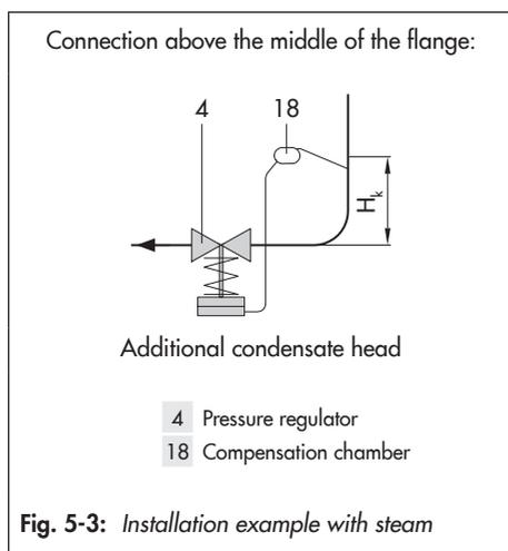
**Fig. 5-3: Installation example with steam**
